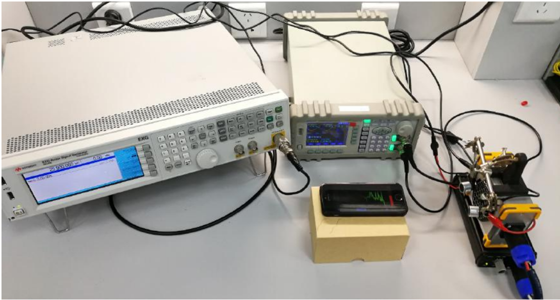
Figure 20: Our benchtop equipment to carry about the proof of concept reproduction of tones heard in Cuba. Note, we would expect emitters to be smaller than a paperback book in practice, if not smaller. We use large equipment because of our general-purpose laboratory.
